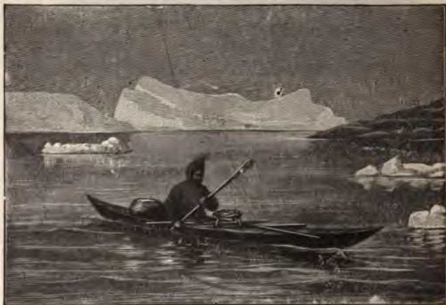
FIG. 387. A Greenland Eskimo in his boat ( Kayak ). It is a canoe made of skins sewed together over a light framework of wood. In this light canoe, using a harpoon, he kills seals, walruses and so forth.
